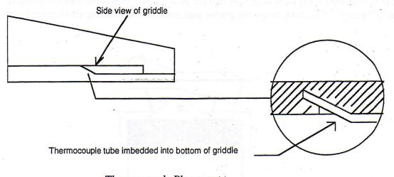
Thermocouple Placement Figure 5
